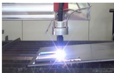
AVC function test in an extreme condition. Smooth height control is achieved on 4-degree angled plate.
