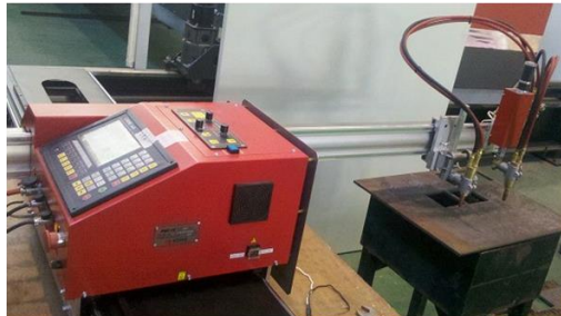
Secondary oxy-fuel torch mounted on the cross bar.
