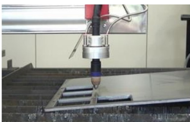
AVC function test in an extreme condition. Smooth height control is achieved on 4-degree angled plate.
