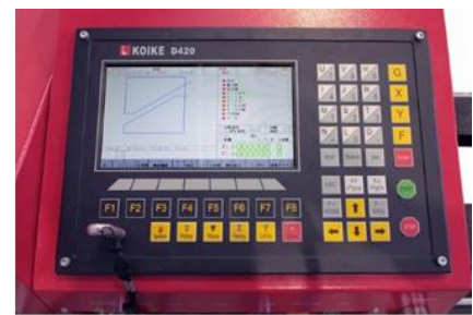
By importing NC data from USB, virtually every shape can be cut with PNC-12 Extreme.
