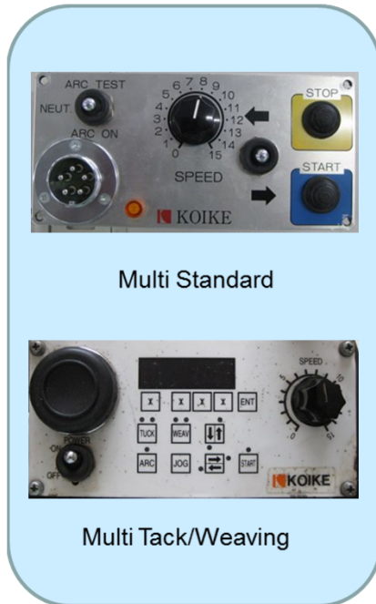
Current operation panel
