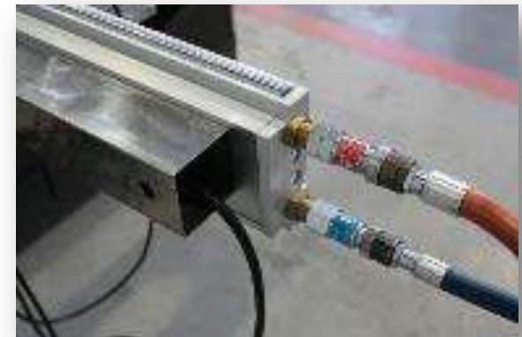
Gas hoses are connected at the end of cross bar (quick-connection couplings are optional)
