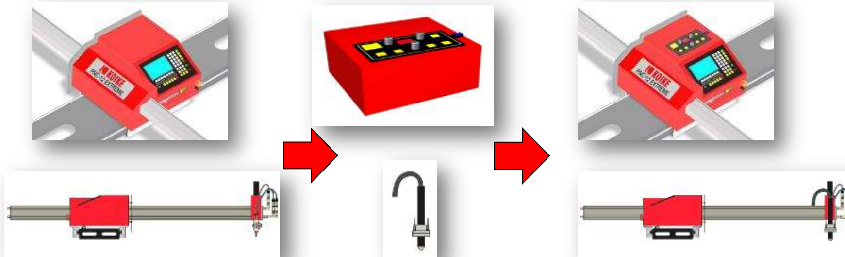
Mount plasma torch unit and signal cable. Oxy-fuel related units and signal cable need to be dismounted completely.
