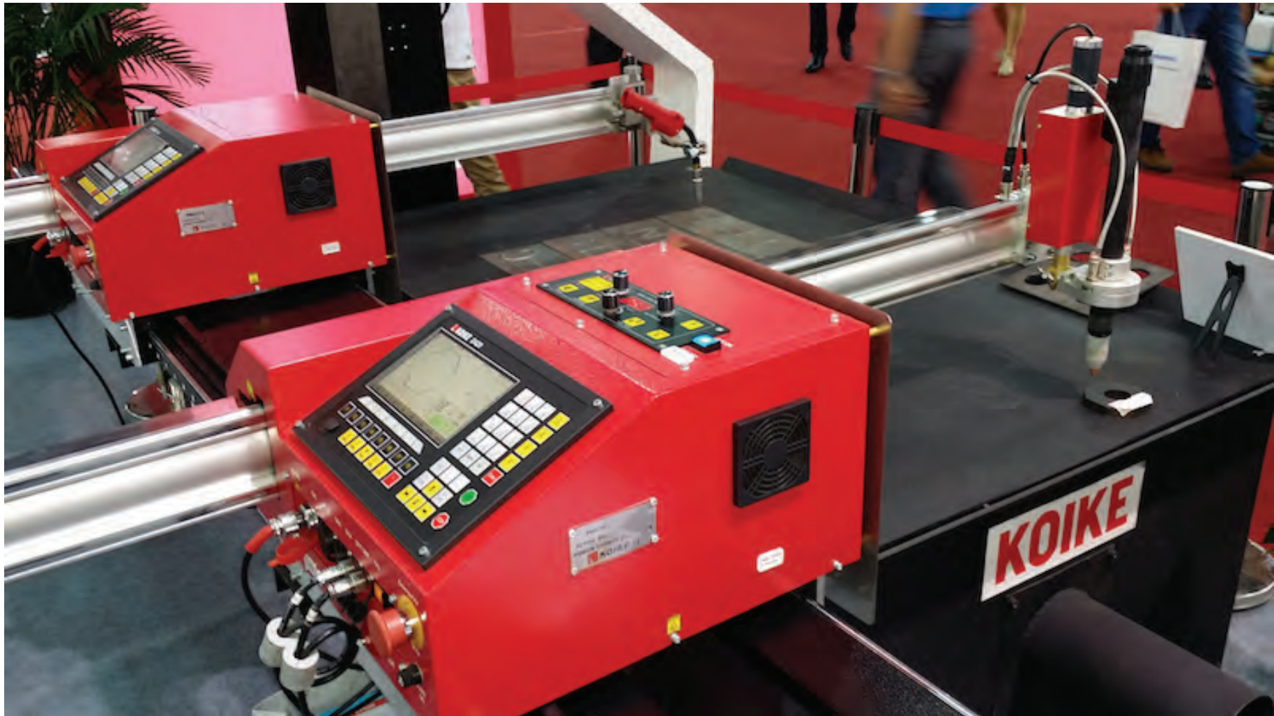
KOIKE PNC 12 WELD & CUT – Rail track can be extended for longitudinal profile cutting.
