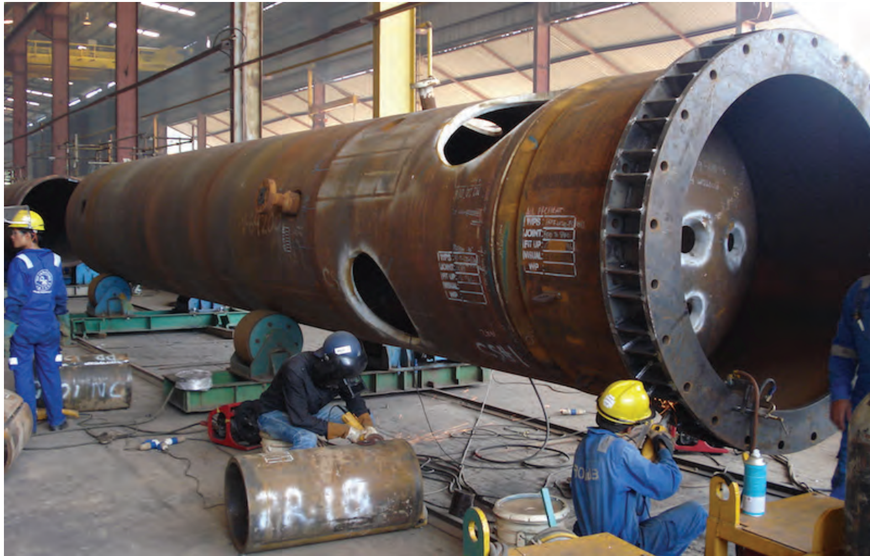
KHC 600D pipe hole cutter is excellent for nozzle hole cutting on large vessels.
