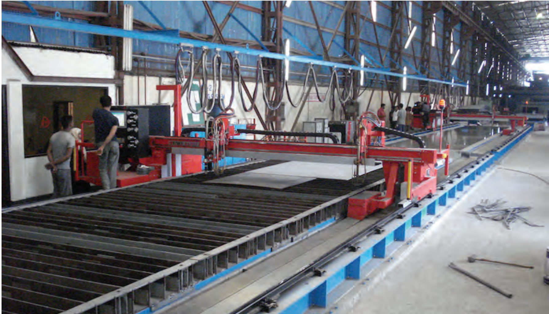
KOIKE MAXIGRAPH 4500 DD – D500 – MAX 200 Plasma & Gas cutting system. Courtesy of Ananda Shipyards – Bangladesh.
