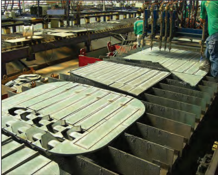
CUTTING OF PARTS FROM SCRAP.
