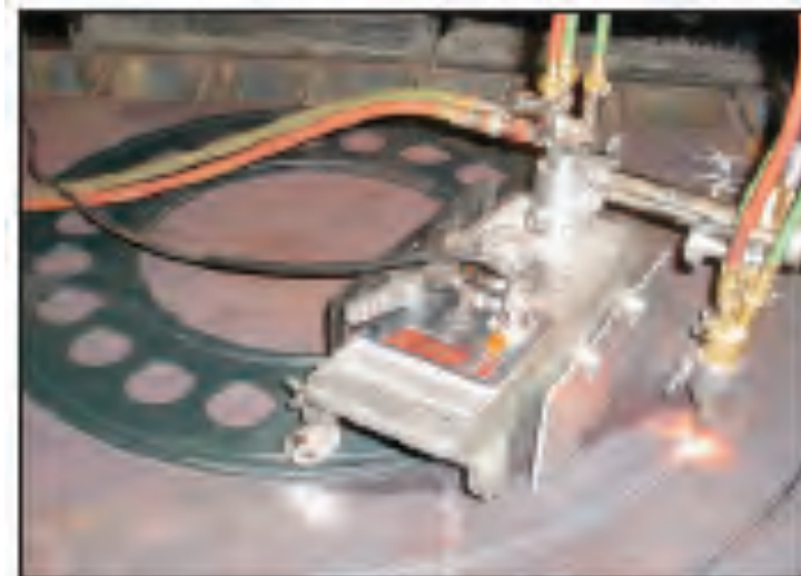
Using IK12 Beetle with circle track. Inside cutting range : 40 - 360 mm Outside cutting range : 770 -1150 mm
