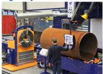
The SPC-RB is equipped with a logistic system. To further improve productivity, different in-feed and out-feed systems are optionally available.
