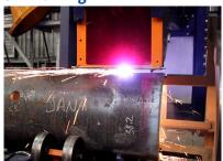
The SPC-RB is equipped with a patented biaxial cutting head that can be used to cut with both oxyfuel and plasma.
