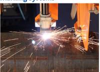
The machine can be equipped with plasma (above), inkjet or punch marking for traceability and easy fit-up, ensuring the lowest fitting times.
