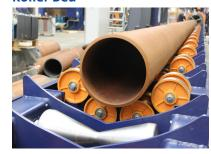
A roller bed is used as pipe support. Tandem wheels prevent vibrations during cutting (e.g. due to weld seams) and guarantee accurate cuts.
