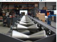
To even further improve the productivity of the RBPC, it can optionally be equipped with an in- and out-feed system. This will improve and speed up handling time of the pipes.
