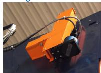
The optional marking system can even further improve your productivity. The RBPC can be equipped with punch, ink-jet or plasma marking systems.
