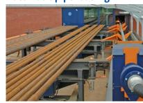
The large pipe buffer allows the loading of multiple pipes (bundle) at once. The infeed of pipes into the cutting cell occurs fully automatically.
