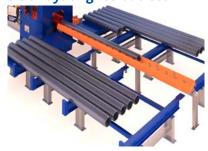
The sideways aligned outfeed configuration sorts parts on sloped tables adjacent to the outfeed gutter so that they roll to the far end.
