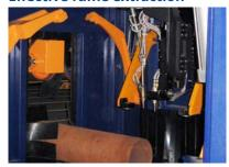
Achieved by use of a cutting cell. Fumes generated inside the pipe will be extracted through the main drive.
