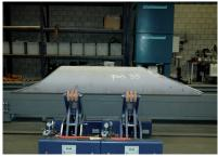
The SPC is equipped with adjustable pipe supports to level he pipe at cut location. These hydraulic pipe supports have coated wheels and a scissor mechanism to enable handling bow shaped pipes.
