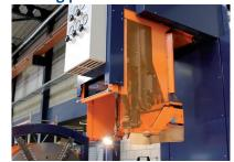
The SPC is equipped with a patented biaxial cutting head to perform 3D cutting routines highly accurate with both plasma and/or oxyfuel cutting processes.
