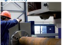
The self centering three jaw chuck is one of the factors influencing accuracy. It achieves high accuracy by clamping pipes securely, avoiding slip and creep (longitudinal movement) during rotation.
