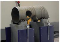
The ProCutter is equipped with adjustable pipe supports to level he pipe at cut location. Furthermore, the ProCutter can be equipped with a rollerball gutter that provides permanent horizontal support.
