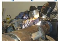
HGG pipe profiling machines practically eliminate the need for grinding, so that fitting time is greatly reduced. These factors apply in the same way to the welding process.
