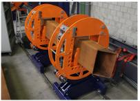
Both pipes and box sections are cut on the same supports. However, to easily rotate box sections, HGG has developed a special rotator with easy loading from the top.
