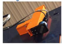
Optionally, a marking system can even further improve your productivity. The MPC can be equipped with punch, ink-jet or plasma marking systems.
