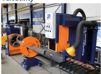
The MPC is available in several possible configurations. Depending on customer requirements, the machine is able to cut (a combination of) pipe, box section and/ or flat bar.
