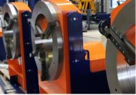
A 4-jaw chuck is used to clamp both pipes and box sections. Pipes and box sections are rotated very precise, resulting in highly accurate cuts and less grinding afterwards.
