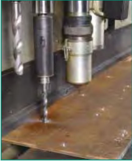
Multiple spindle drilling, countersinking, and similar operations can be achieved.
