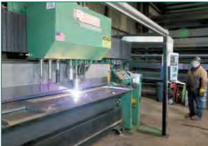
Punch, drill, thermal cut via plasma or oxy/fuel, and mark in one operation.
