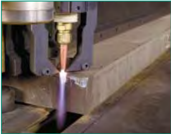
The Oxy/Fuel torch delivers CNC accuracy on 3" (75 mm) thick plate.
