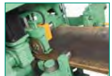
Continuous throughput via Roller Feed technology.
