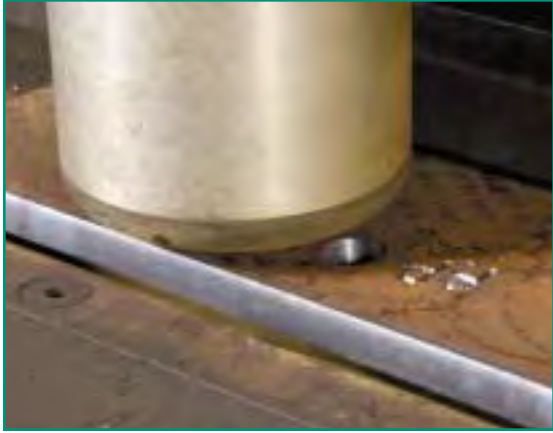
The Signoscript Scribe Marking System employs a milling cutter for easy piece part identification to any height or depth.
