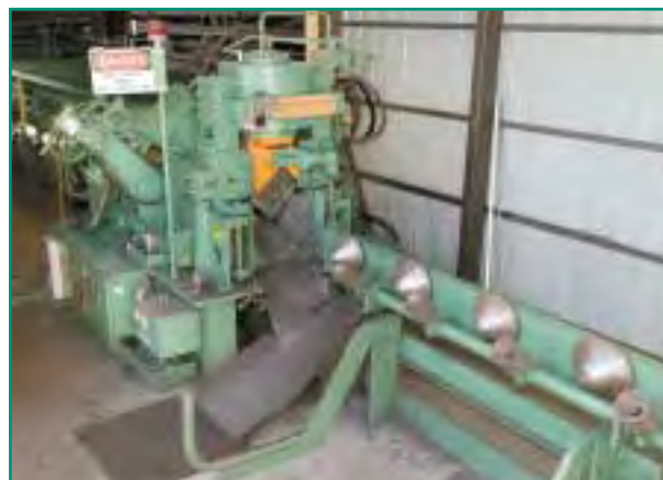
Combining the technologies for punching (130 tons/118 metric tons) and shearing (400 tons/363 metric tons) with an automated loading and unloading system saves not only labor, but material handling costs as well.
