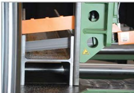
Saw profiles with a 7° attack angle
