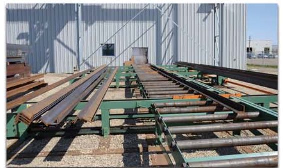
Cross transfers and Roller Feed systems can be stored outside for loading.
