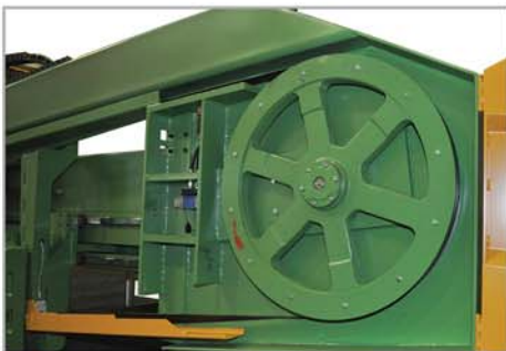
The large diameter blade wheel requires less bending of the blade resulting in a longer blade life
