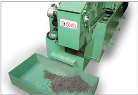
Automatic chip conveyor for streamlined maintenance
