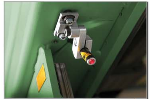
Laser reference for precise cutting
