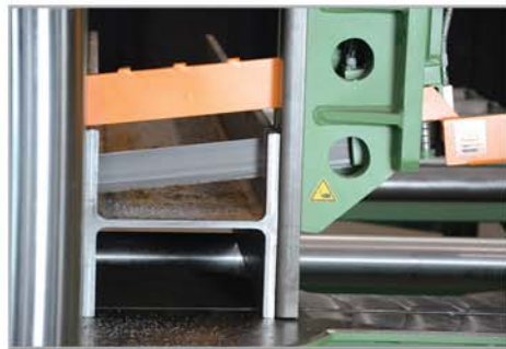
Saw profiles with a 7° attack angle
