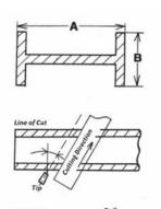
The **Mini-Mantis II** provides high-precision diagonal cuts that are clean and sharp. Two motors drives the torch for both web and flange cutting. No need to turn and mark the workpiece.
