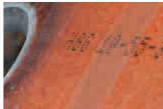
Marking for traceability and easy fit-up.
