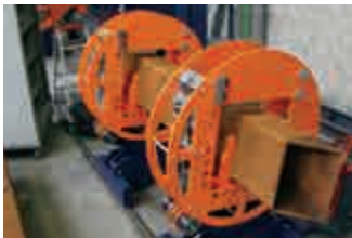
Box section support HGG has developed a special rotator with easy top loading.
