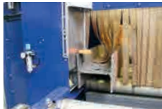
Ink or punch marking to mark text on the flange.
