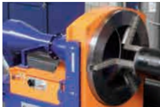
High precision chuck for pipe centring and accurate rotation.
