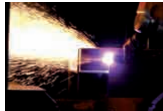
Plasma cutting for rapid cutting without the need of pre-heating.
