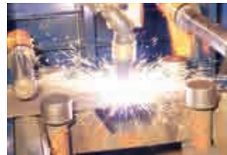
Plasma cutting to cut carbon steel, alloys and even aluminium.
