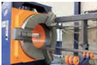
Heavy duty precision chuck for pipe centring and accurate rotation.
