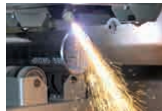
Oxyfuel and/or plasma cutting to cut carbon steel or alloys.
