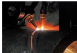
Oxyfuel or plasma cutting to cut carbon steel or alloys.
