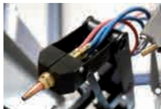
Compact cutting arm to perform 3D cutting routines.
