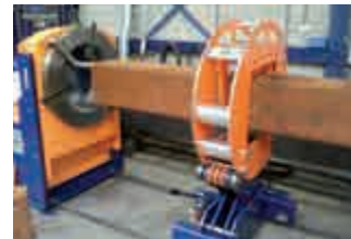
High precision chuck for material centring and accurate rotation.
