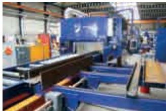
Conveyors and buffer tables allowing fully automatic material handling.
