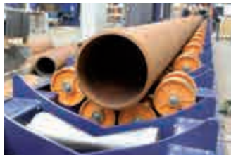
Tandem wheel sets to level pipe at cut location and allow out-feed during cutting.
