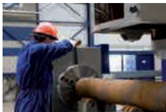
3-Jaw chuck for pipe centring and accurate rotation.
