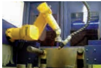
Compact robot arm moves dynamically with the gripper during plasma cutting.
