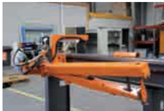
Material gripper For exact material positioning in linear direction.
